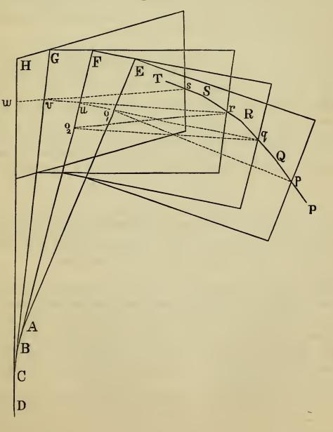
Through p let a plane be drawn perpendicular to PQ and through  $q, r, s \dots$  planes perpendicular to  $QR, RS, ST, \dots$ respectively. These will ultimately be normal planes to the curve at consecutive points. Let the planes through p, qintersect in a line AE, and the planes through q, r in a line BF which cuts AE in some point A, and so on.
